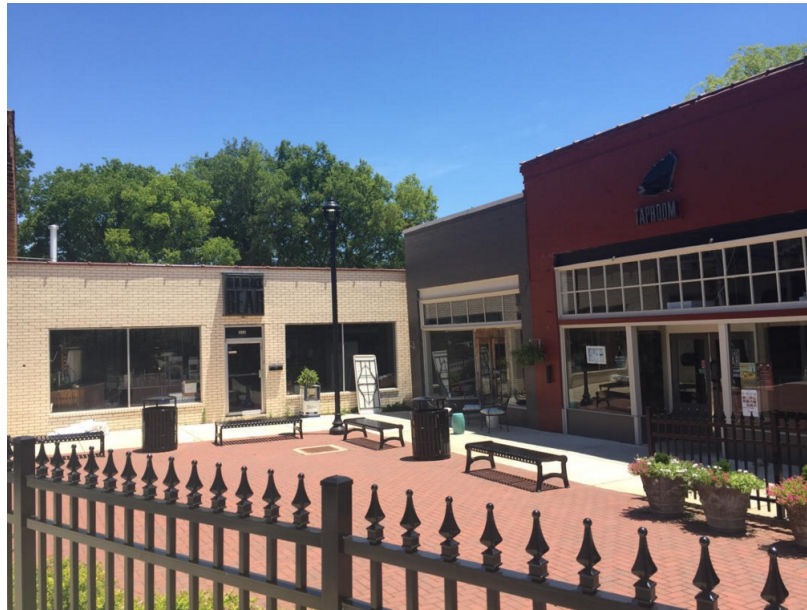
Figure 1107-B: The above is an image provides an example of facade transparency with the use of windows and glass doors along the facade that provide for visibility of at least four feet into the building.
