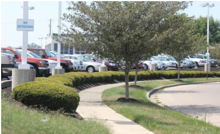
Figure 1119-A: The above image illustrates an example of the provision of a two-foot-high landscape barrier along the street right-of-way, adjacent to the sidewalk.
