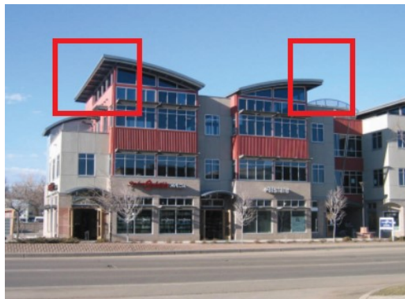
Figure 1117-F: Example the use of eaves, highlighted in red rectangles.
